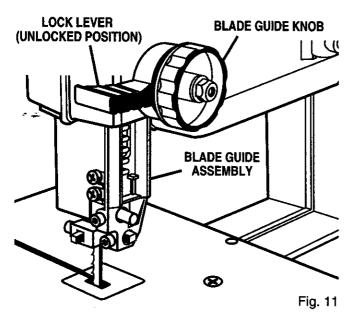
cut as a guide to set the height of the blade guide assembly.
